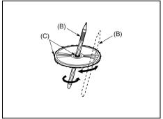
New discs may have some roughness around the edges. The unit may not work or the sound may skip if such discs are used. Use a ball-point pen (B), etc. to remove the roughness (C) from edges of the disc before insertion inside the unit.
